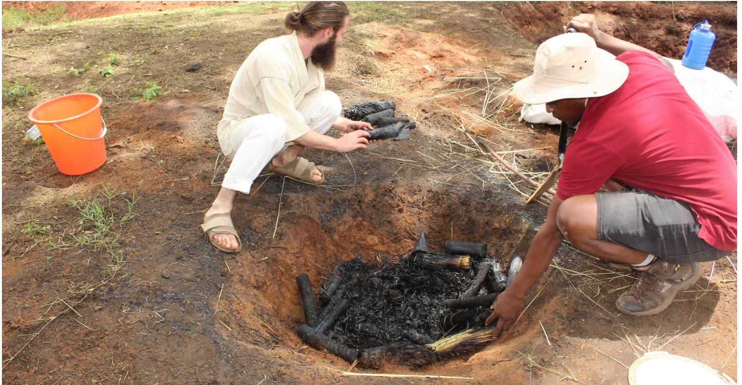
CarbonConnect co-founder Nando Knodel and OFA biochar consultant, Tafadzwa Nyamande demonstrate how to produce biochar using a cone-shaped pit at CIMMYT-Zimbabwe premises .
